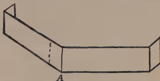
Fig. 267.—The pasteboard is now ready to be tacked on to box-making pointed end.
